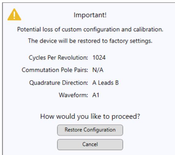
Figure 14: Restore Factory Configuration Warning
