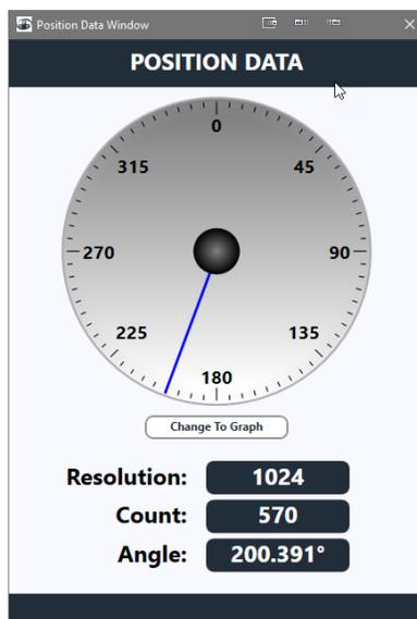
Figure 16: Position Data Detail w/ Radial Gauge
