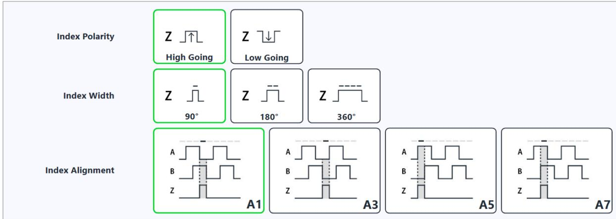
Figure 12: Waveform Selection
