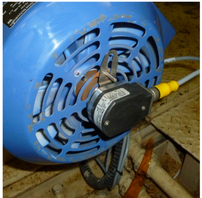
A compact, 2-inch blind hollow bore encoder (1) provides motion feedback on a motor. The flex mount (2) stabilizes the encoder, and the cable sends the electrical signal to the receiver.
