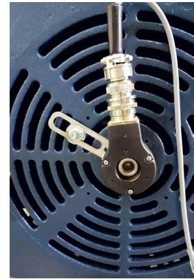
An EPC Thru-Bore Encoder in a common application, mounted on a motor with an SJ Flex Mount
