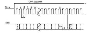
The encoder data bits are sent MSB to LSB, with multi-turn position bits sent first (if applicable), followed by single-turn position bits.
