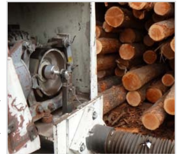
A Model 25T with an SJ Flex Mount Arm mounted on a motor shaft (inspection panel removed). In its harsh outdoor environment at a lumber mill, the dust-tight IP66 seal also protects the encoder from outdoor moisture.
