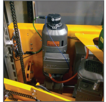
Model 25H encoder mounted on a motor
