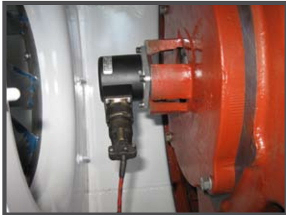
An EPC Size 25 Encoder in a common application
